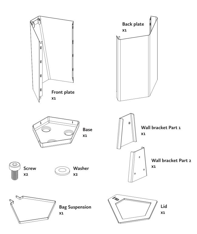
**Kite Mini Floor:** The wall brackets (part 1 and 2) are not included. **Kite Mini Wall**: Wall Brackets are included. The frame is prepared with holes for installation, right or left hung.
