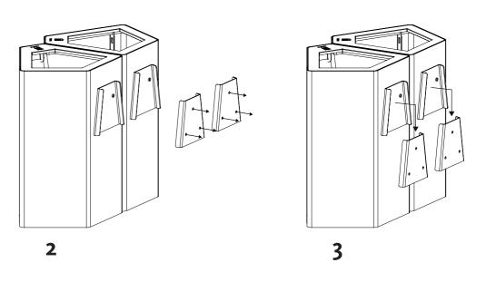
Note that the hole spacing differs depending on whether it is left- or right hung.
