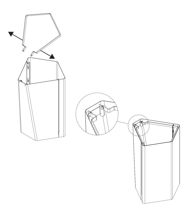
Bend the open ends of the bag holder apart and place the holes onto the cylinders that are attached to the top of the front plate.
