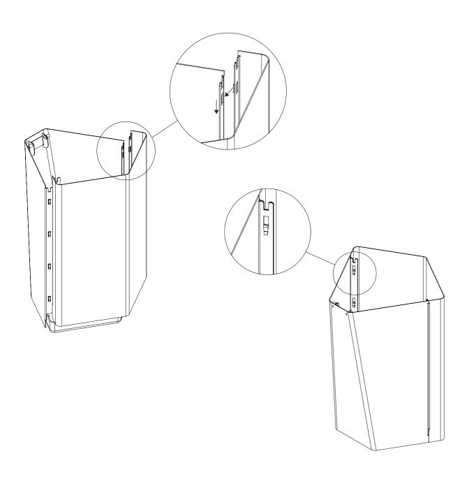
Attach the front and back plates to each other by inserting the sides of the back plate so they fit into the front plate's hole spacing. Make sure the top edges align.
