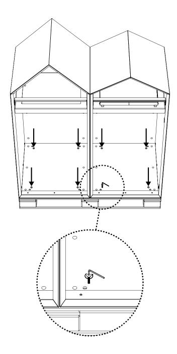
To release the product (s) from the pallet: Unscrew the transport screws (4 screws in each product) using the included allen key (4 mm).
