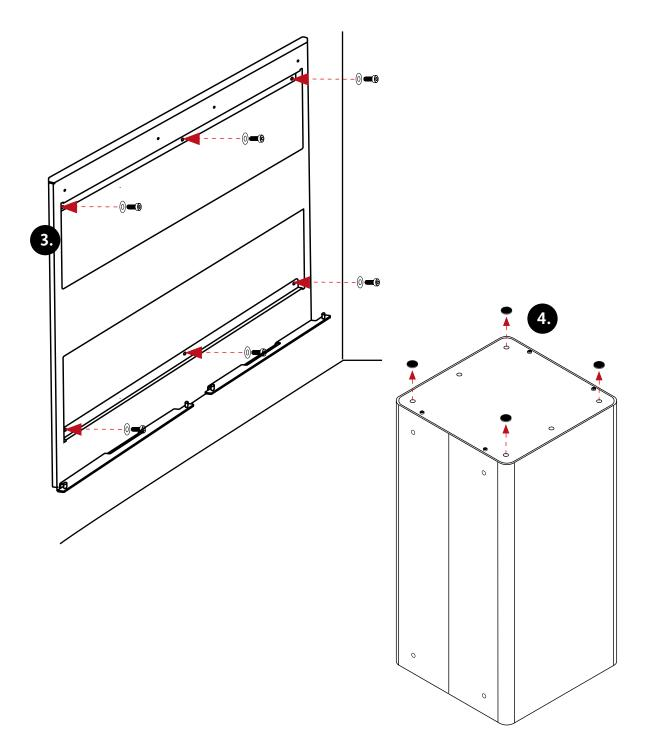
**3.** Mount the wall bracket with screws that are adapted to the chosen wall. **NOTE!** Screws for the wall are not included.
