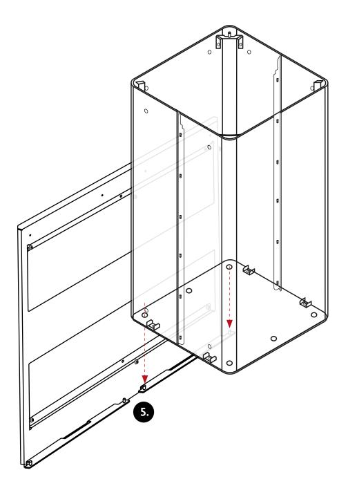
**5.** Place the KLOSS frame on the pins of the support strip. The studs fit the hole pattern of the base plate.
