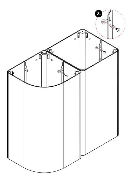
8. Lock the frame parts together in the designated holes with screws, washers, and nuts for additional stability. DONE!
