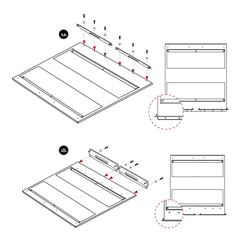
Lay the wall bracket down and screw the support strip into the 3 threaded holes at the bottom with the supplied screw, the tabs on the support strip should be facing upwards. Repeat if it is Wall mount 2 or 3.
