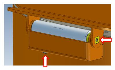
8. Screw on the washer and Allen screw. Check that the lid opens easily and that it dampens when closed.
