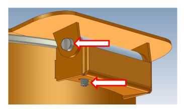
3. Using a small tool, push in the square socket about 10 mm, be careful not to damage the threads. Remove the lid and lift up the damper unit.
