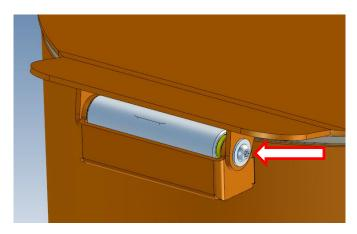
2. Loosen the bottom stop screw half a turn with a 3 mm Allen key, then unscrew the groove screw on the side.
