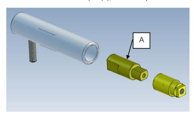
5. Replace the damper with the new one, attach the square socket to the damper and reinsert it into damper unit. Make sure that the larger key grip on the damper comes parallel to the stop screw. The smaller key grip on the damper should be about 90° to this. This is set at the factory and cannot be changed.
