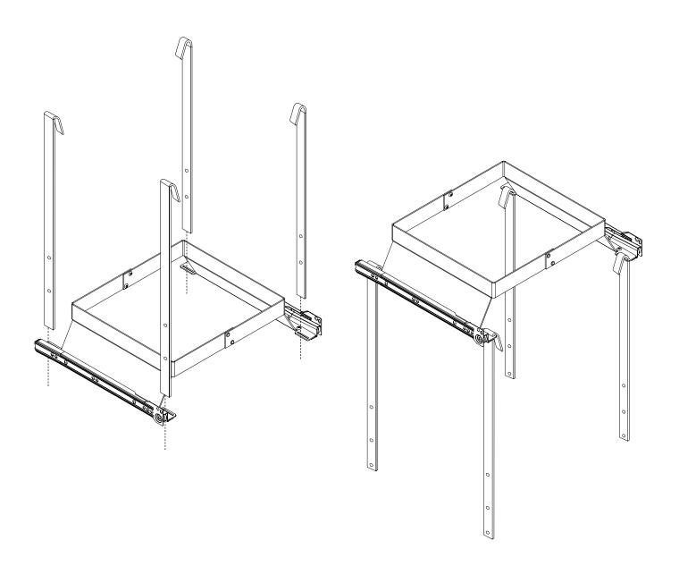
Insert the braces into the holes on the frame, according to the picture.
