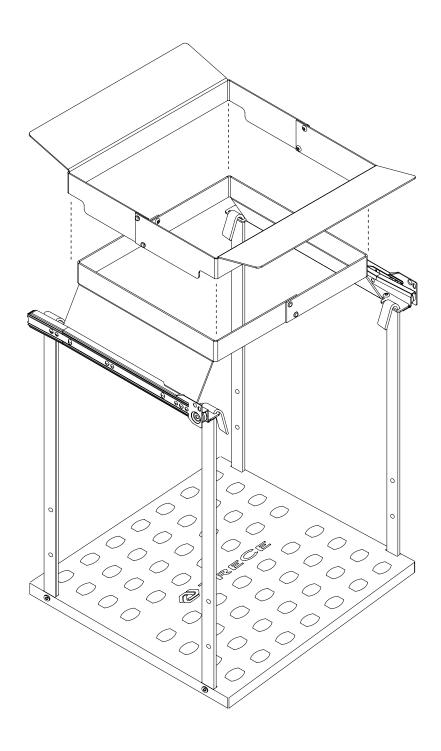
Fix the garbage bag with the clamping ring as shown in the picture.
