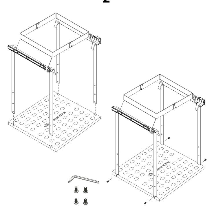
Screw the base plate to the desired height on the struts and hang it inside Cloud.
