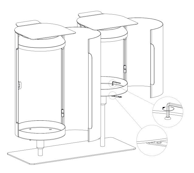
After the bin/bins are centered, tighten all the screws in the base of the bin/bins.
