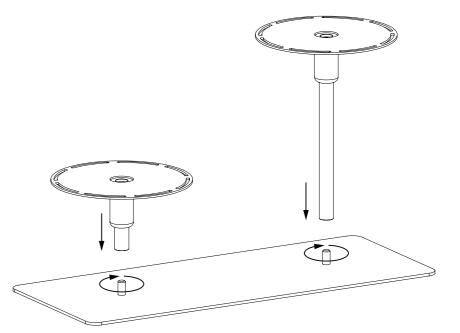
Adjust the bin/bins so that they are centered with the front edges of the lids parallel to the long side of the foot plate.
