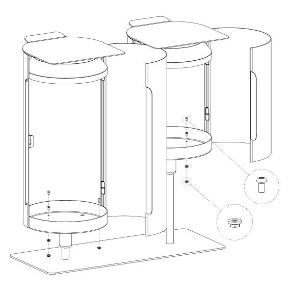
The bin/bins are screwed onto the plates with the supplied screws (3 per bin).
