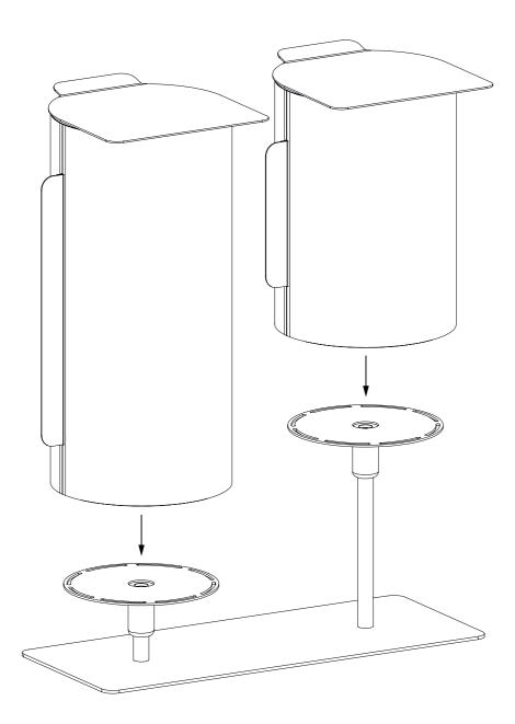
The bin/bins are lifted onto the circular plates at the upper ends of the shafts.
