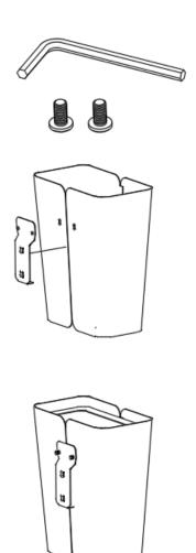
Mount the wall bracket with 2 screws from inside the bin.
