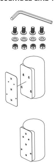
Mount the wall bracket with 4 screws from the outside, washers and nuts from the inside Tork M1 dispenser (not included)
