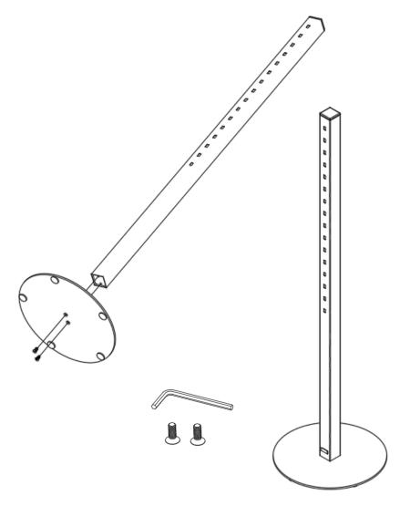
Mount the stand on the foot with 2 screws, tighten.
