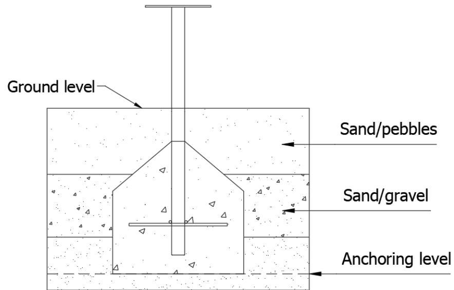
When the foundation has hardened, fill the cavity in the hole with sand / grit to the ground surface, like instruction shows. Place the Popsicle on the mounting plate.
