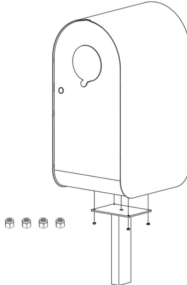
Then mount the bin on the foot plate with 4 nuts and a U-ring 10-key (tools not included)
