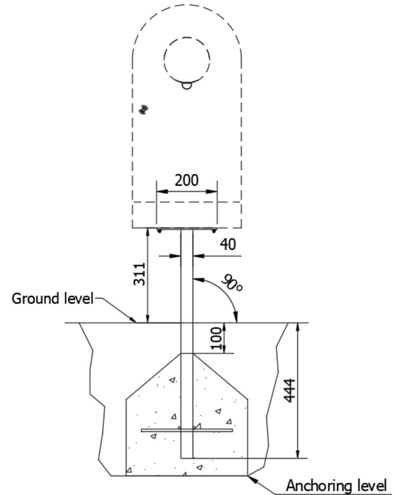
Dig a hole where Popsicle is to be placed to a frost-free depth, minimum depth 550 mm. Fill with stones/pebbles at the bottom. Place the leg at the correct height and cast a concrete foundation in the hole, the mounting plate should be 311 mm above ground level. NOTE! The narrow part of the leg should be forward and the mounting plate horizontal. Let harden.
